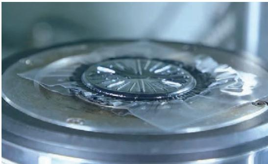
We determine the time and heat required for the vulcanization and also the properties of the rubber by conducting a Rheometer test.
