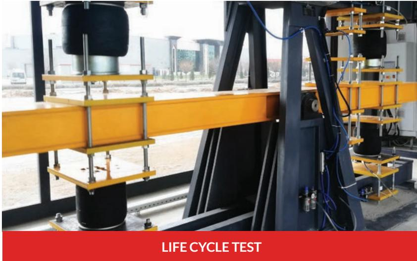
Wisgroup performs lifecycle tests at 7 Bar and 3.3Hz.
