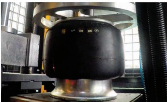
Although the working pressure of the vehicles is 7 bar, our products meet the pressure standard of 21 bar min, which is 3 times higher.
