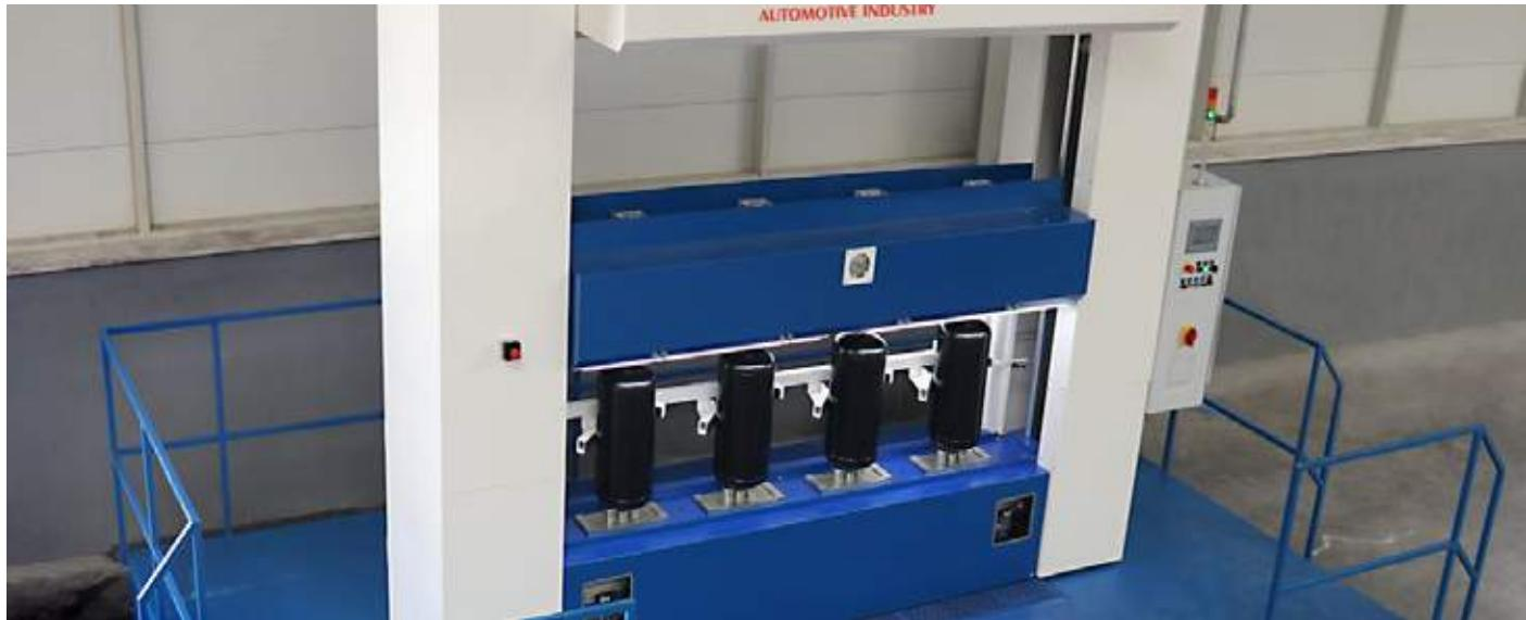
We are doing 100% high pressure tests to all our products as specified in the CE directives. We always prioritize product and vehicle safety and test the sealing and compressive strength of the each products cylinder, cover and sleeve surfaces under the test conditions which are 1.5 times higher then the maximum working pressure ( $P_s = P_{max} \times 1.5$ ).
